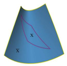
Fig. 11. A rational Bézier surface X (with purple boundary curves) contained in another rational Bézier surface  $\overline{X}$  (with yellow boundary curves). The reparameterization of X can be done by trimming a parameterization of  $\overline{X}$  using the boundary curves of X. (For interpretation of the references to colour in this figure legend, the reader is referred to the web version of this article.)
