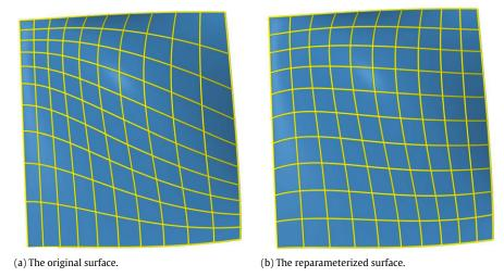
**Fig. 4.** A rational bilinear reparameterization of a rational Bézier surface: (a) the original Bézier surface and its parameterization; (b) the reparameterized Bézier surface and its parameterization with the reparameterization coefficients  $\alpha_1 = 0.69$ ,  $\alpha_2 = 0.34$ ,  $\beta_1 = 0.36$  and  $\beta_2 = 0.40$ .
