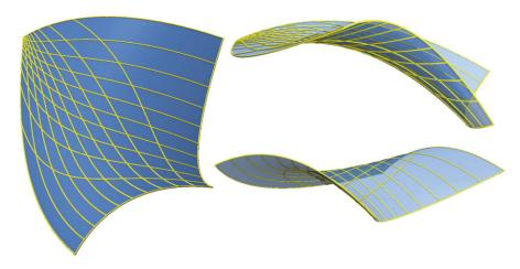
Fig. 7. Three different views of the second surface and its parameterization.
